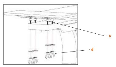
Note: before fully tighten "d", please move the extension marble more left or right, or adjust "c" to make it more up or down so that the extension can be aligh with the middle marble well.
